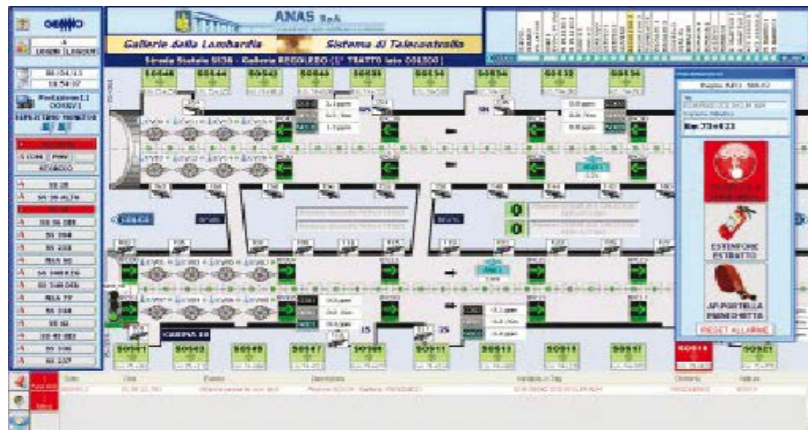
Fig.4 - Main page with alarms and info window for the Regoledo tunnel
