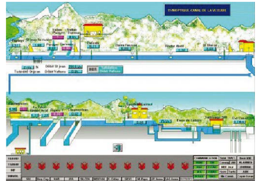
Mimic panel representing a drinking water pipeline feeding into the Super Rimiez plant
